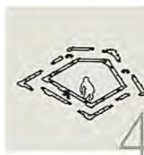
4 Set out the parts for each section onto the ground, assembling it like a jigsaw.
