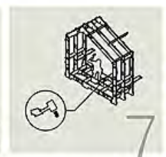
7 Fit the connector pieces into the slots in the section. These should be staggered
